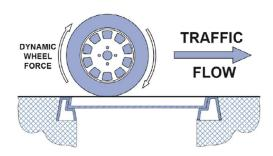
To prevent covers lifting, position covers such that traffic flow direction is from undercut to drawcut.
