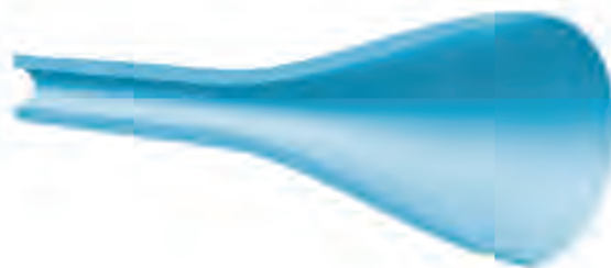
Figure 1.5: Wall cross-section of “pre-form” pipe with a small diameter and a large wall thickness being stretched circumferentially and axially into a pipe with larger diameter and a thinner wall.
