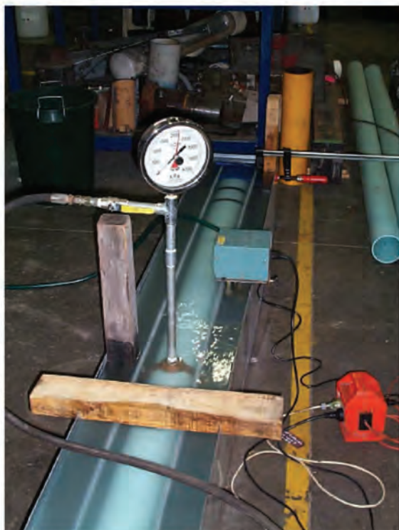
Figure 7.14: Testing a gunmetal tapping band installed on ApolloBLUE™ as part of a comprehensive evaluation in accordance with AS/NZS 4793.
