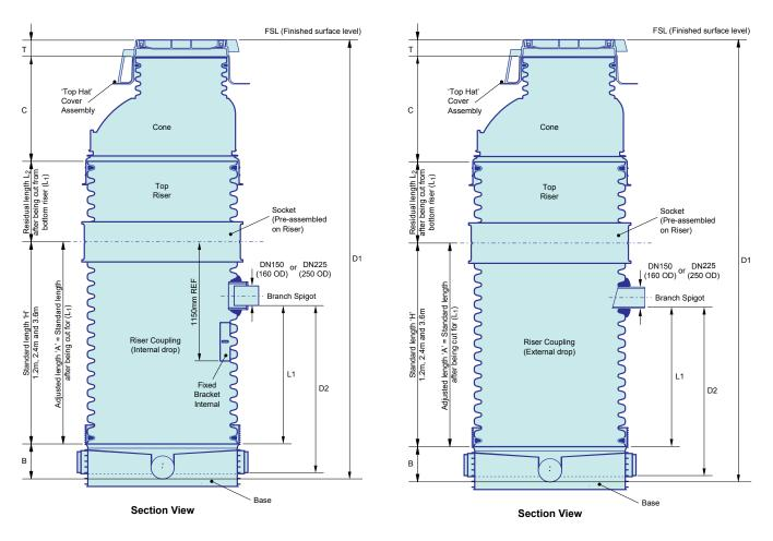
Figure 55: EZIpit® 1000 MH Assembly with Riser Junction (Branch Connection)
