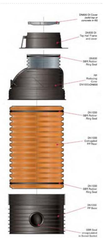
Figure 44: EZIpit® 1000 Maintenance Hole (MH) assembly
