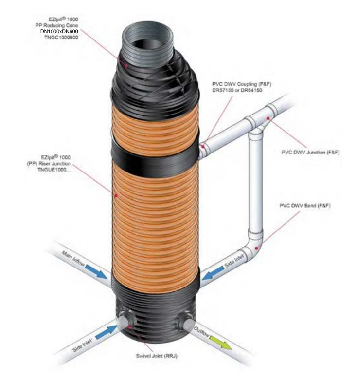
Figure 51: EZIpit® 1000 Maintenance Hole (MH) with external drop structure
