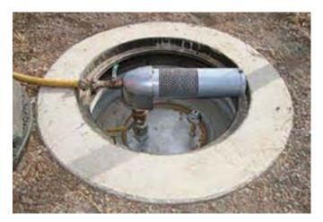
Figure 16: Vacuum test with EZIpit® test Lid assembled on the Cap and sealed with GATIC® Sealing Compound.
