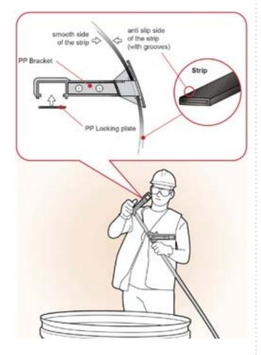
O2 Position the assembled lower ladder support (assembled strip and brackets) in the groove of the Riser. Refer to Table 11 Column 6 for correct location of the lower ladder support. Ensure the joint on the Strip is positioned directly opposite the ladder. I.e. at 180° to the ladder
