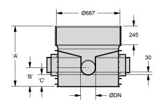
Note: Side inlets with slight slope (1°) and sockets positioned 30mm higher. No fall through the main flow channel.
