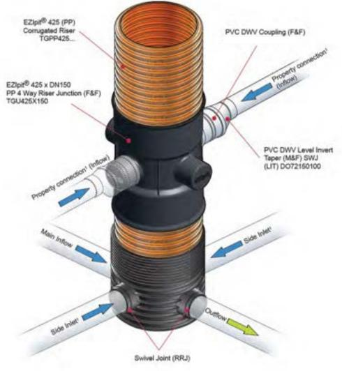
Figure 26: EZIpit<sup>®</sup> 425 Maintenance Shaft with lateral sewer connections via the base and the riser.
