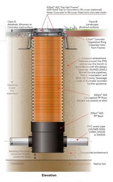
Figure 27: Typical Installation EZIpit® 425 Maintenance Shaft (MS).
