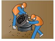
ring. Remove the lid from the cap and apply GATIC<sup>®</sup> sealing compound liberally to all vertical and horizontal seating surfaces of the lid and assemble on the cap.
