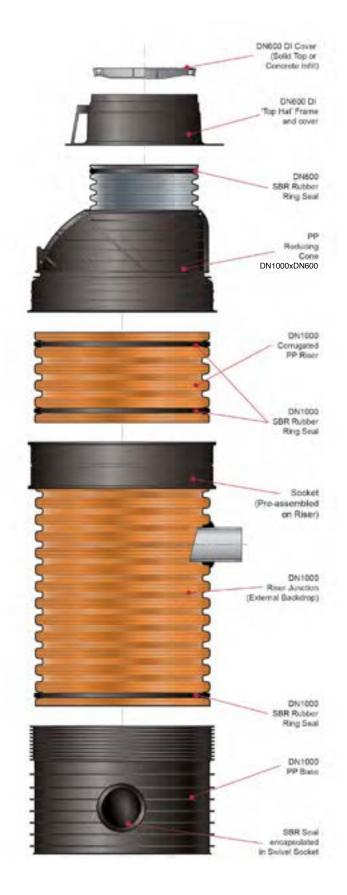
Figure 52: EZIpit® 1000 Maintenance Hole (MH) assembly with Riser Junction for External Drop
