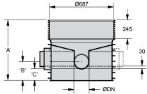
Note: Side inlets with slight slope (1°) and sockets positioned 30mm higher. No fall through the main flow channel.
