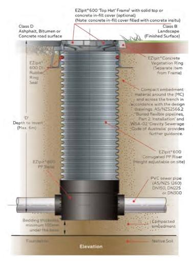
Figure 39: Typical Installation EZIpit® 600 Maintenance Chamber (MC).
