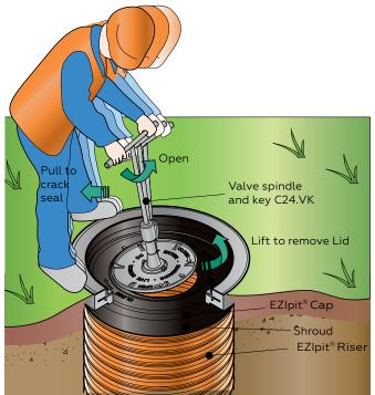
Figure 17: Removing the EZIpit<sup>®</sup> Lid from the Cap for Sewer Inspection or Vacuum Testing.
