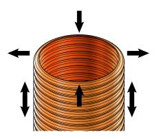
Figure 7: The flexible nature of the EZIpit<sup>®</sup> corrugated riser allows a robust structure.
