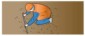
**O2** Position the base on the bedding material with a spirit level. Apply Iplex pipe seal lubricant to the pipe spigot and base socket seal for ease of assembly. Connect the base to the pipe by pushing it onto the pipe spigot end.
