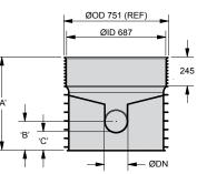
ØDN150 = 160mm OD PVC Smooth Wall DWV pipe ØDN225 = 250mm OD PVC Smooth Wall DWV pipe ØDN300 = 315mm OD PVC Smooth Wall DWV pipe
