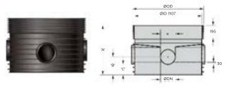
ØDN150 = 160mm OD PVC smooth wall DWV pipe ØDN225 = 250mm OD PVC smooth wall DWV pipe ØDN300 = 315mm OD PVC smooth wall DWV pipe
