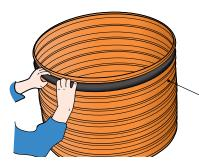
**O9** Apply Iplex pipe seal lubricant on the inside of the base socket and push the riser down (with the sealing ring) into the base socket. Ensure the riser is kept perpendicular to the socket.
