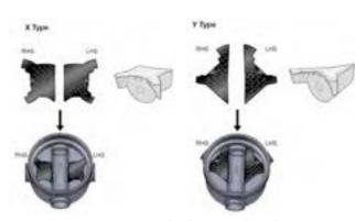
Note: TNGPLUG...200's are used with DN1000xdn150 bases. TNGPLUG...300's are used with DN1000xdn225 & dn300 bases.
