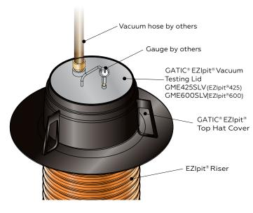
Figure 19: Vacuum Testing using DN425 or 600 GATIC° EZIpit° Lid with 'Top Hat' Frame.
