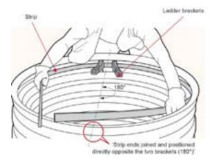
**03** Bend one leg of the ladder Strip to help locate the two ends of the strip in the riser corrugation. The male and female ends of the strip must engage in the valley of the corrugation. Press down on the bent leg until the strip 'clicks' into position.
