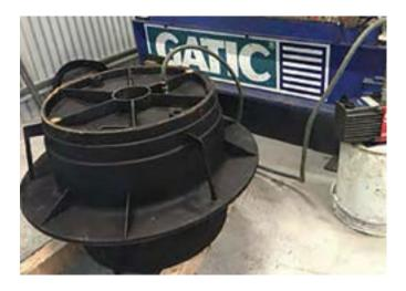
Figure 8: GATIC<sup>®</sup> EZIpit<sup>®</sup> 600 'Top Hat' Cover under vacuum test.
