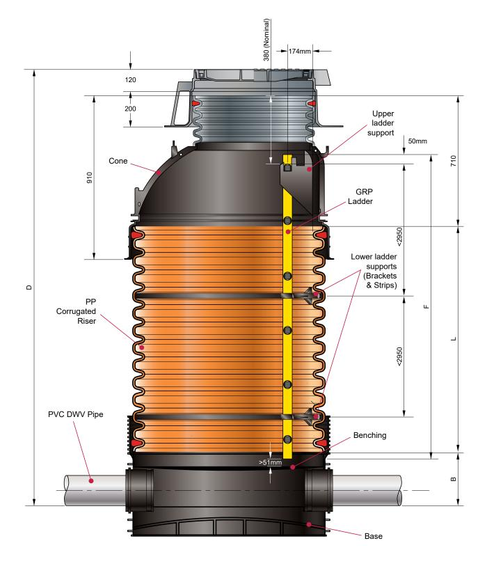
Figure 61: EZIpit® 1000 MH with ladder and critical dimensions
