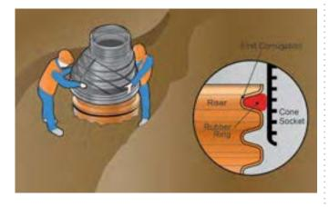
Backfill the trench and around the cone with embedment material. Ensure even coverage around the cone up to the surface. The embedment should be compacted in layers not exceeding 300mm. Large and sharp stones should be removed from the surrounding area to avoid damage to the cone.
