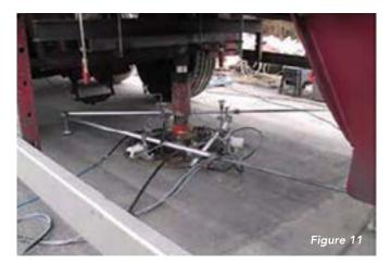
The robust, tough, ductile nature of the EZIpit<sup>®</sup> riser is demonstrated in the 'run over' test. The riser did not crack or break under the extreme loads encountered on site. (Figures 13, 14 and 15).
