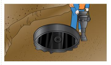
**07** Use the corrugated riser to build up the maintenance hole. Cut the riser to the required length (refer to 'field height adjustment' Sections 5.5 and 5.6) with a circular saw or handsaw. Cut the riser at the top of the corrugation or in the valley. Remove swarf.
