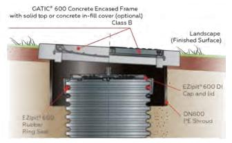
Figure 40: EZIpit<sup>®</sup> 600 Cover arrangement (sloped surfaces).
