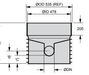
ØDN150 = 160mm OD PVC smooth wall DWV pipe ØDN225 = 250mm OD PVC smooth wall DWV pipe
