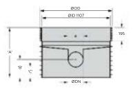
ØDN150 = 160mm OD PVC smooth wall DWV pipe ØDN225 = 250mm OD PVC smooth wall DWV pipe ØDN300 = 315mm OD PVC smooth wall DWV pipe
