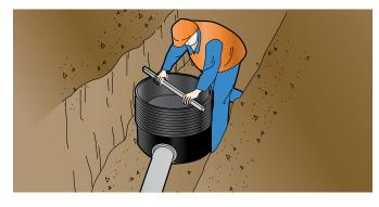
**O3** Adjust the pipes to the required position. The adjustable pipe connector enables an angular deflection of 7.5° from the centre line in all directions.
