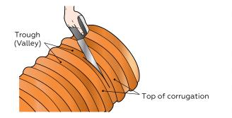
**08** Assemble the sealing rings in the 1st valley at each end of the riser. Ensure the sealing ring is sitting correctly in the valley of the corrugation.
