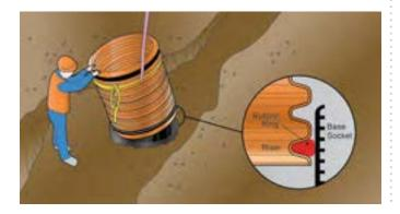
**10** If the riser height needs to be raised use a double socket with two additional rings. For this type of joint the riser should be cut on top of the corrugation on both sides.
