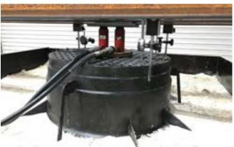
Figure 12: EZIpit<sup>®</sup> 1000 MH under load in accordance with ISO Standard 13266
