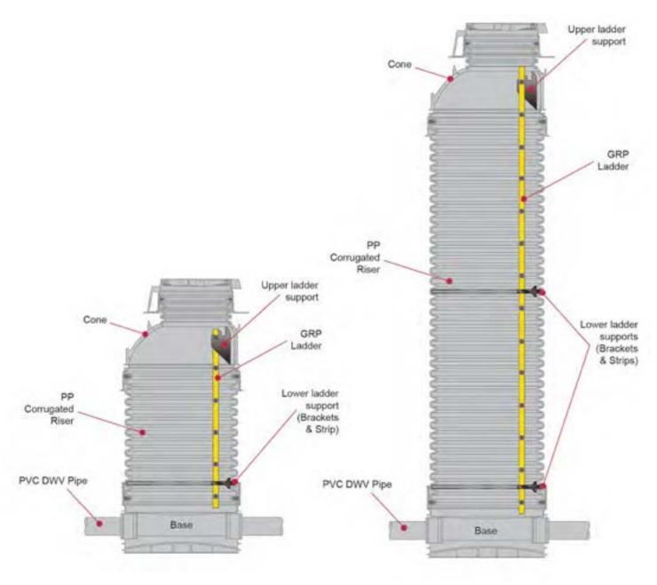
Figure 56: EZIpit<sup>®</sup> 1000 MH ladder with one lower ladder support. (Maximum installation depth 3.671m)
